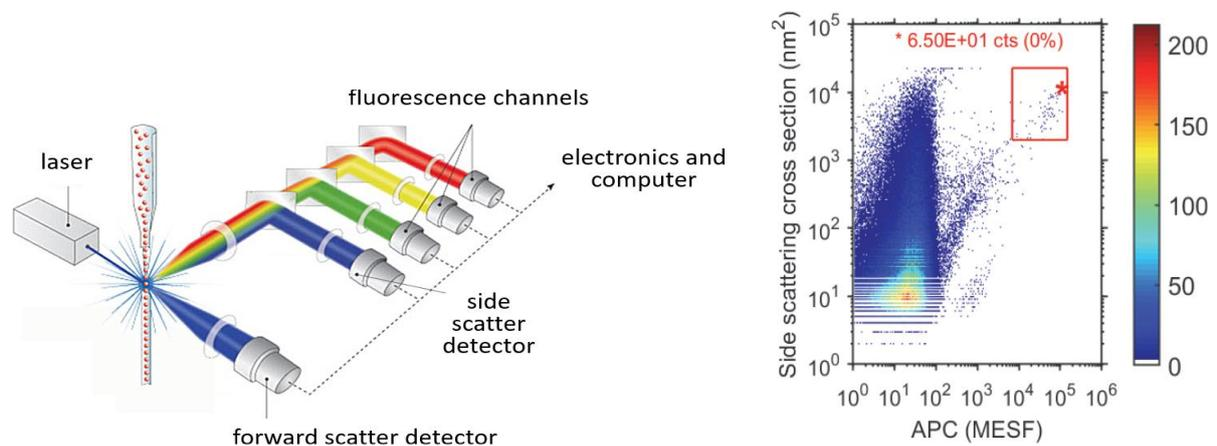
Figure 1. Left: schematic representation of a flow cytometer. Flow cytometry detects light scattering and fluorescence signals of hundreds of thousands of extracellular vesicles (EVs) per sample. Right: snap-shot of a typical flow cytometry dataset of EVs.
