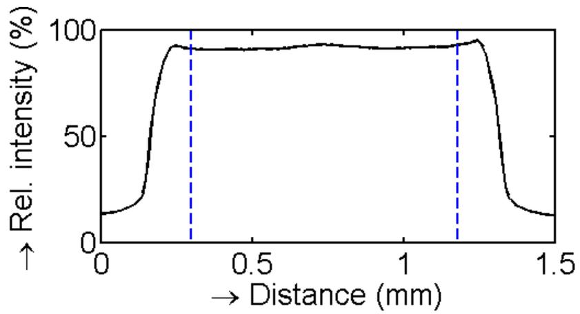
**Figure S3-2. Line profile of a well aligned MLA system, with correctly xy aligned arc lamp.** The profile is shown in the long direction of the arc, some residual asymmetry is due to the shape of the arc.
