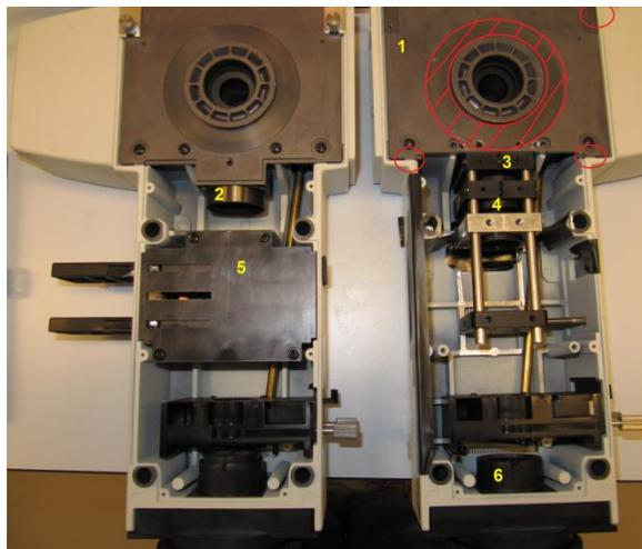
**Figure S3-1. Modification of Nikon Eclipse 400 epi fluorescence module.** Steps needed for modification of this module shown in yellow: Plate (1) machined to mount MLA close to filter cube (the surfaced used to mount this piece in the machining vice are shown in
